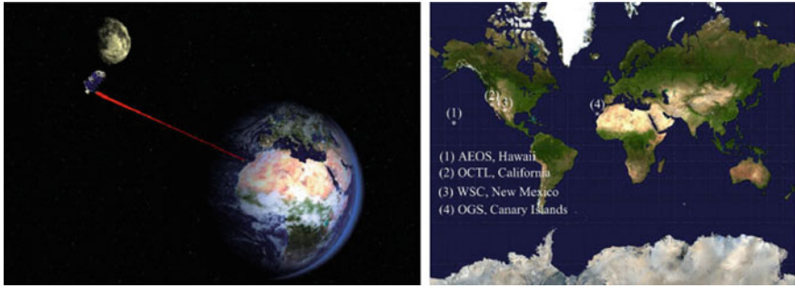
Fig. 18.2 Schematic of the lunar laser communication scenario (left) and the locations of the three ground stations (right)
