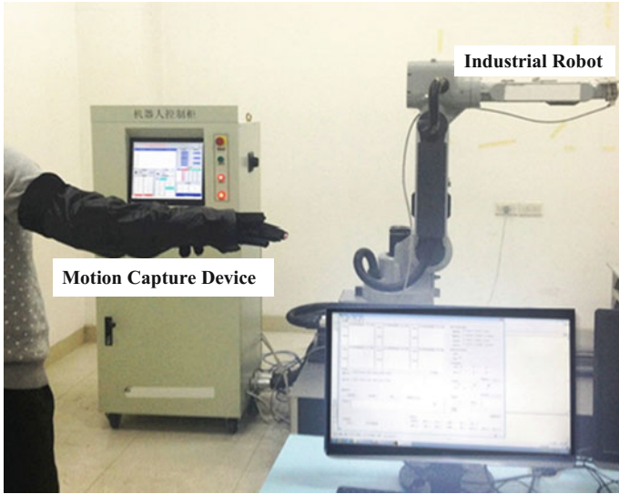
Fig. 21.8 A teleoperation ground experimental system based on human motion capture
