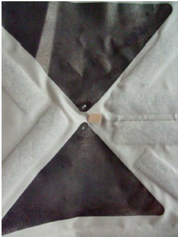
Fig. 6 Copper coated fabric bow tie antenna
