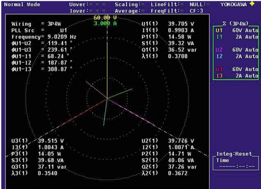
Fig. 9 Practically measured voltage and current vector graph for normal inverter drive
