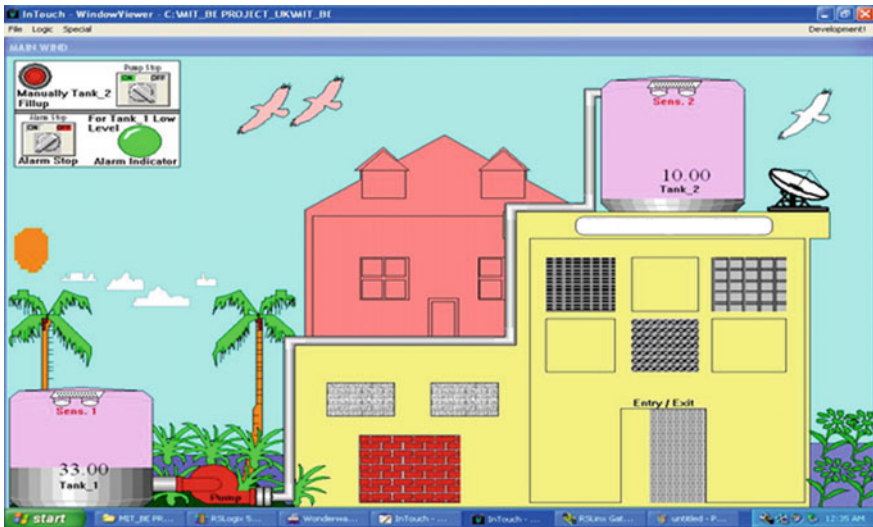
Fig. 10 Alarm indicated as level of water lowers in underground tank
