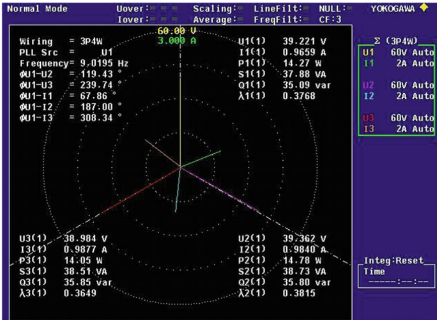
Fig. 11 Practically measured voltage and current vector graph for FCMI drive
