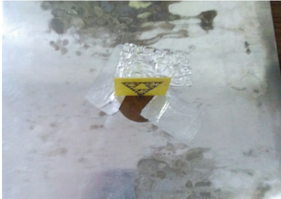
Fig. 5 Sierpinski gasket on rectangular ground plane
