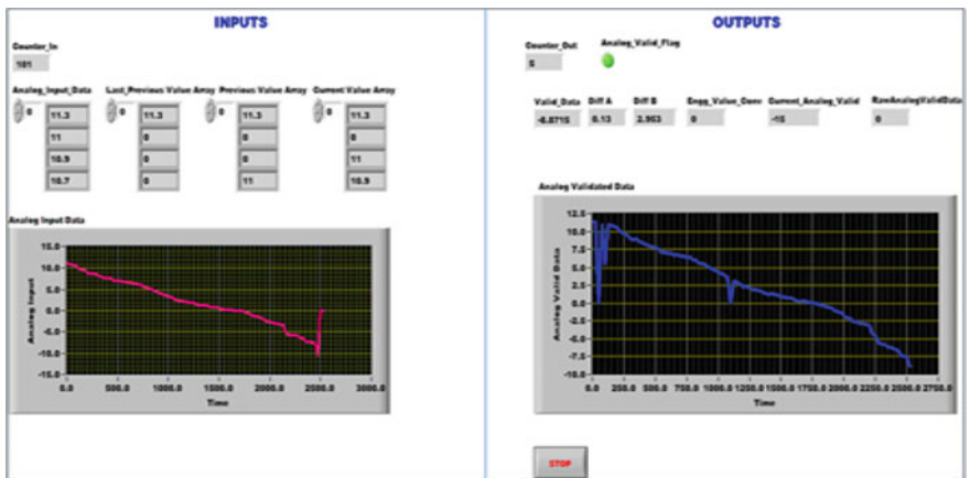
Fig. 9 LABVIEW front panel representation for overall implementation model
