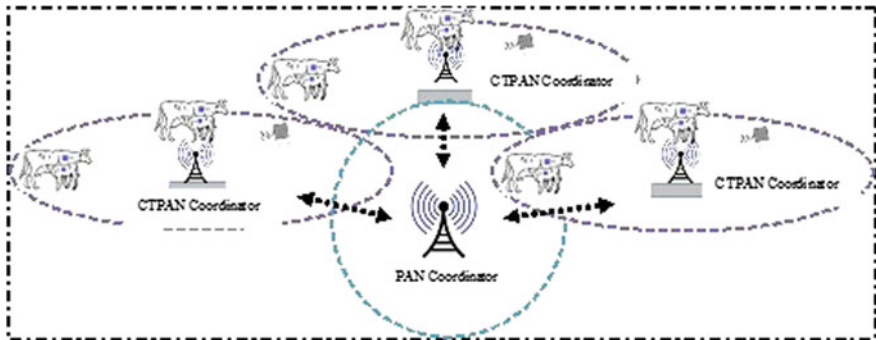
Fig. 1 Proposed architecture of three PAN-based animal shades
