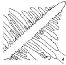
Fig. 2 Simulated dendrite structure and dendrite arm spacing (d) between two arms of dendrite structure [1]
