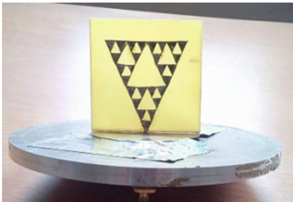
Fig. 6 Sierpinski on circular ground plane
