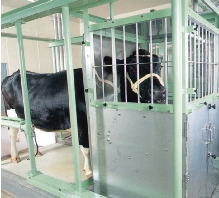
Fig. 12.3 Ventilated hood system for measuring in vivo methane emission
