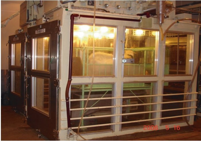
Fig. 12.2 Open circuit respiration chamber for sheep
