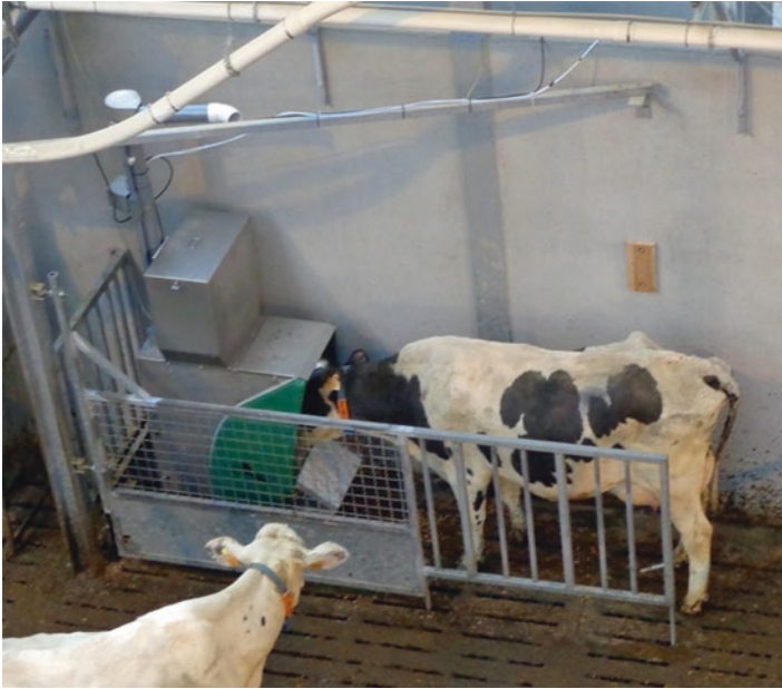
Fig. 12.6 Methane measurement in GreenFeed unit
