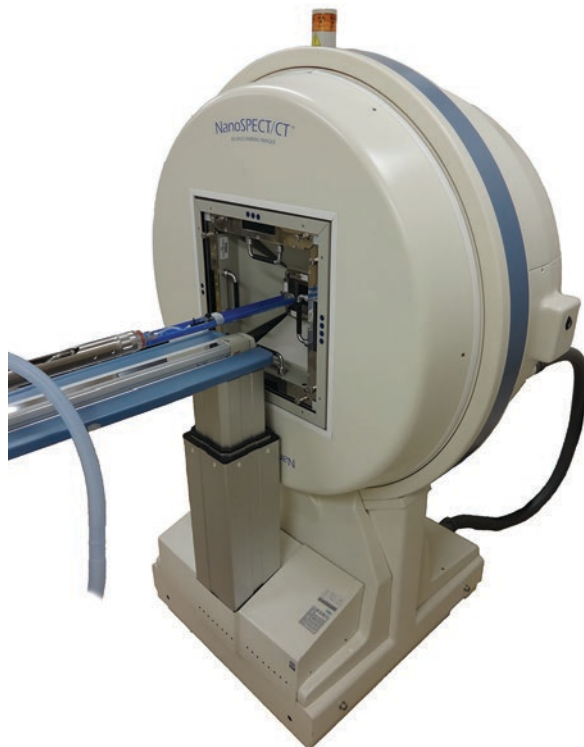
Fig. 6.5 A SPECT/CT combined scanner (NanoSPECT/CT, Mediso, Budapest, Hungary)
