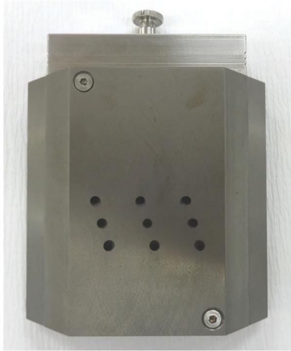
Fig. 6.4 A multi-pinhole collimator for small animal SPECT imaging
