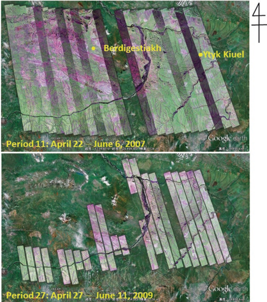
Fig. 5.1 Polarimetric mosaic image derived by PALSAR in periods 11 (April 22–June 6, 2007) and 27 (April 27–June 11, 2009). Red: HH polarization. Green: HV polarization. Blue: VV polarization
