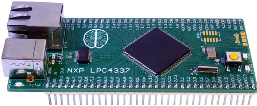
Fig. 6.5 Development board for embedded control based on the ARM ® Cortex ® M4 core
