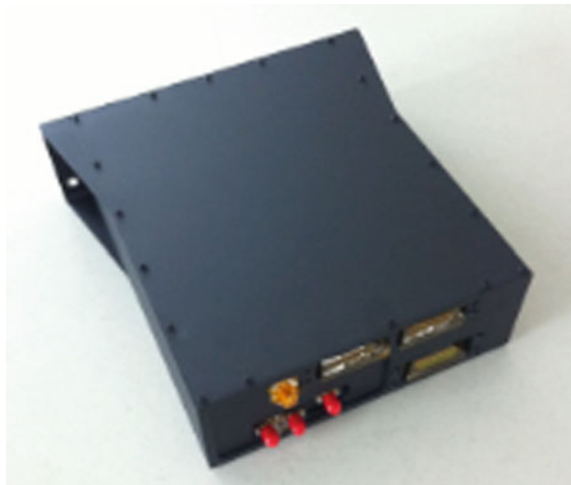
Fig. 1 HiSGR receiver with painted encapsulation
