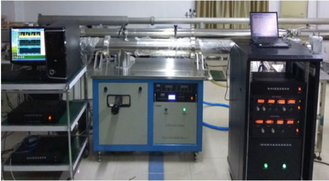
Fig. 1 Hardware in-loop system for X-ray pulsar-based navigation
