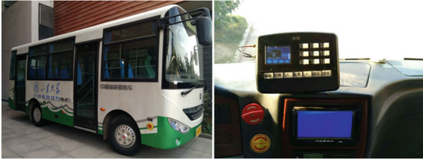
Fig. 4 Experimental vehicle and the intelligent stop device
