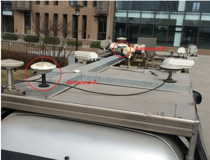
Fig. 3 Antenna configurations in the vehicle experiment
