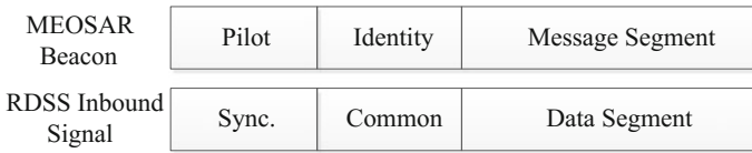
Fig. 2 MEOSAR/RDSS inbound frame structure
