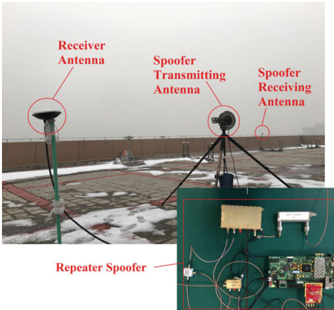
Fig. 4 Meaconing spoofing platform
