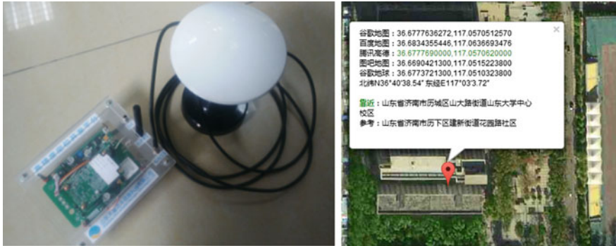
Fig. 3 Handheld locator made with board and the terminal fixed-point test (no differential mode accuracy of 5–10 m)
