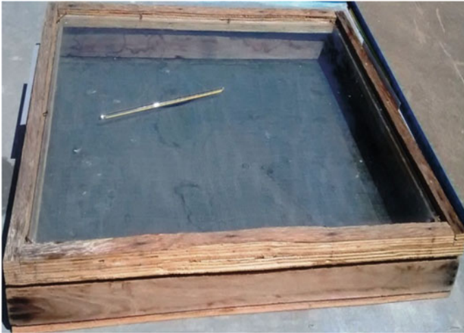
Fig. 1 A low-cost solar dryer developed at CAZRI, Jodhpur
