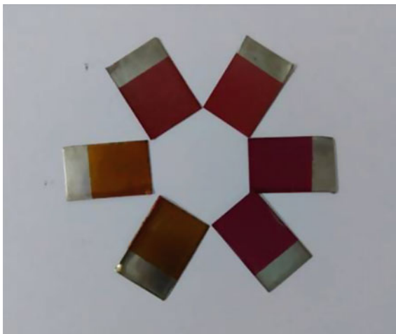
Fig. 2 Optical photographs of spray coated thin films on SS substrates, using transition metals (Fe, Ni, Co and Mn) in ethyl alcohol, heat-treated at 100 °C for 1 h
