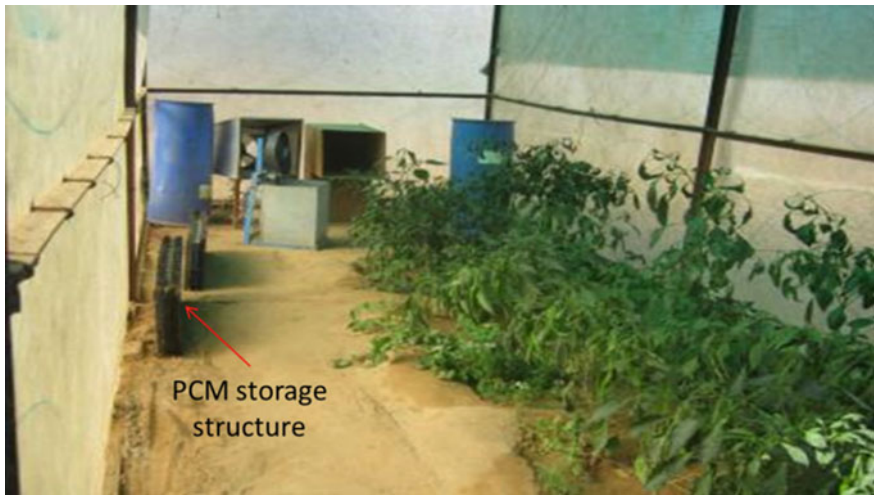
Fig. 5 Experimental trial of PCM material inside protected structure with chilli crop grown inside it
