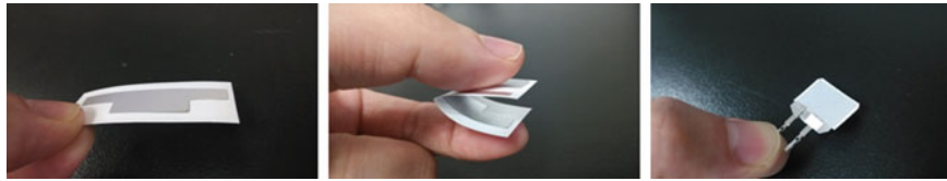
Fig. 1 A flexible piezoelectret film as prepared (left and middle) and a packaged piezoelectret sensor ready for use (right)
