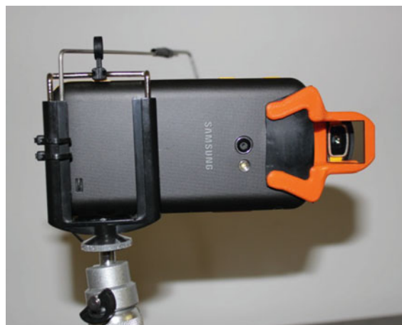
Fig. 2 Smartphone on a small tripod and with a deflection adapter for projectors rays. Note a mirror image of the projector, i.e. a virtual projector
