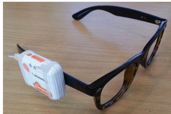
Fig. 1 Setup used for data collection. The Shimmer sensor is firmly attached to the frame using cable ties
