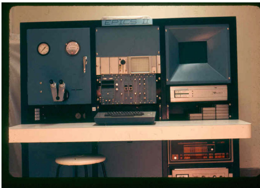
Fig. 11 The SDS-1 sorter developed by Fulwyler and shipped to the NIH in 1974. This instrument had two fluorescence PMTs and a light scatter sensor (0–12 degrees). Its official name was the EPICS II (photo courtesy of Bob Auer used by permission)
