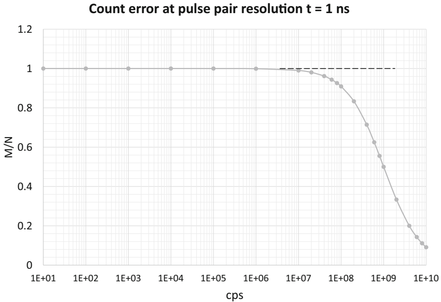
Fig. 3 Calculated count error ratio by photon pulse overlapping at pulse pair resolution 1.0 ns
