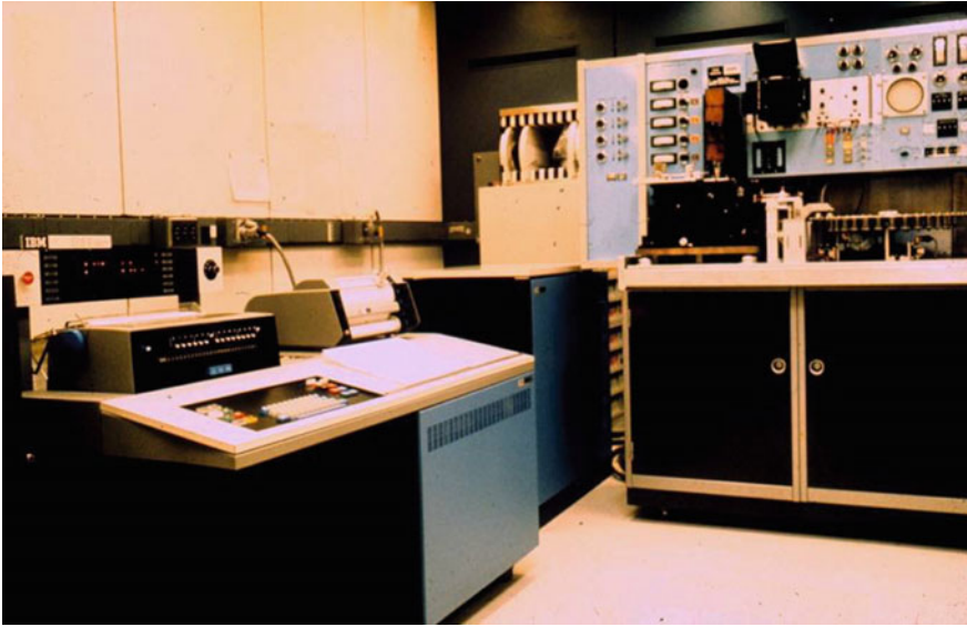
Fig. 8 The 4-parameter cell sorter developed by Lou Kamensky about 1962–1963. Two of these instruments were constructed; one was shipped to the Herzenberg laboratory in 1967 (photo courtesy of Lou Kamensky)
