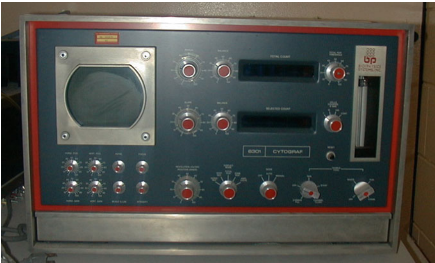
Fig. 9 Kamensky's Biophysics Cytograph. This early-model analyzer measured only light scatter from a red laser. Eventually, a blue laser was added to give the instrument a fluorescence capability and the instrument was renamed Cytofluorograph (photo Copyright J.P. Robinson; used by permission)
