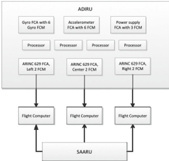
Fig. 2.1 Architecture of the Boeing-777 ADIRU, from [2]
