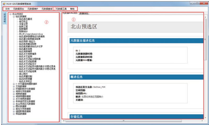
Fig. 3 Metadata management interface: ① Function menu area, ② Data directory list area and ③ Metadata display area
