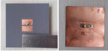
Fig. 3. Photographs of proposed antenna element. (a) top view of the antenna. (b) bottom view of the antenna.
