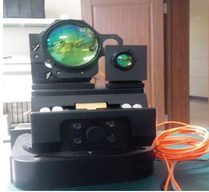
Fig. 11. Laser light wireless transmission system prototype
