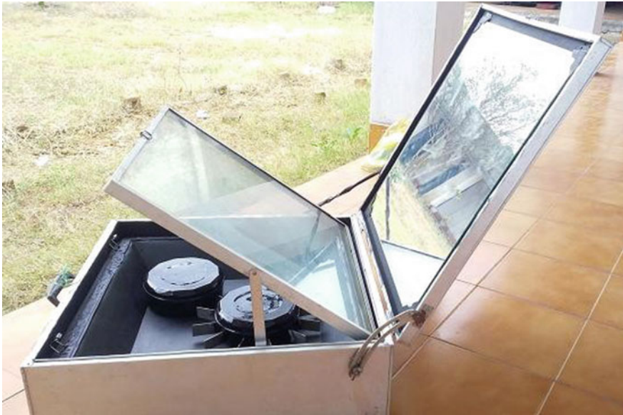
Fig. 1 Constructed box-type solar cooker with pots
