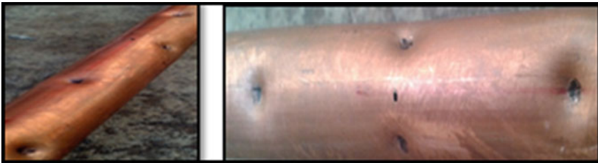
Fig. 2 Dimpled protrusions on the copper tube
