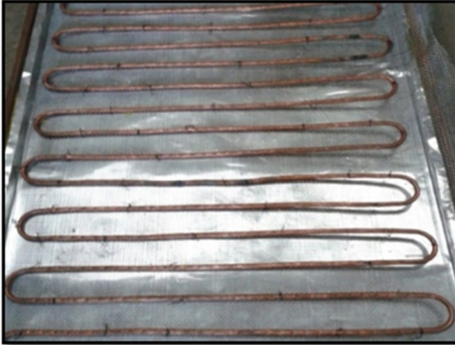
Fig. 1 Arrangement of copper flow tubes for water flow
