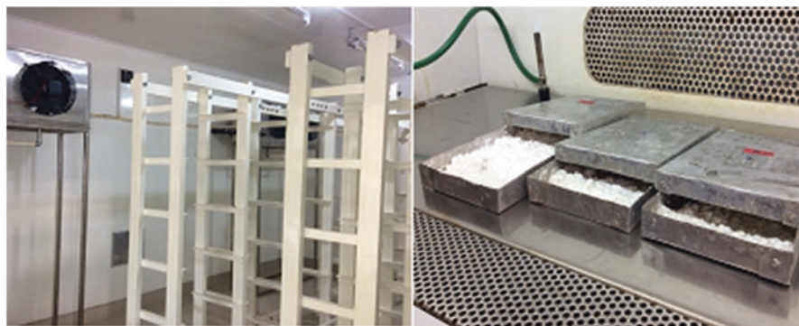
Fig. 1.7 Solid-State Fermentation Facility (Koji) Room (Courtesy – CSIR-NIIST, Trivandrum, India) Koji Room (SSF chamber) showing steel racks for keeping trays and climate control system. Trays showing fully grown Penicillium janthinellum culture ready for harvest (for cellulase production)
