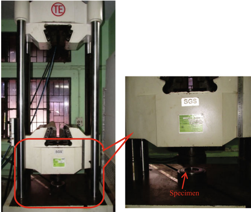
Fig. 2 Experimental set up for uniaxial compression of gasket specimen
