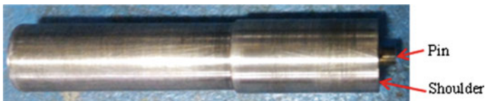
Fig. 1 FSW tool made of H13 tool steel
