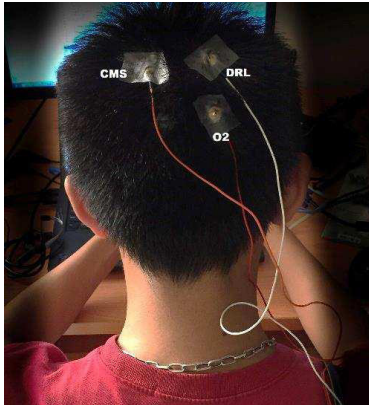
Fig. 3. Electrode placement for comparison with Biosemi's ActiveTwo
