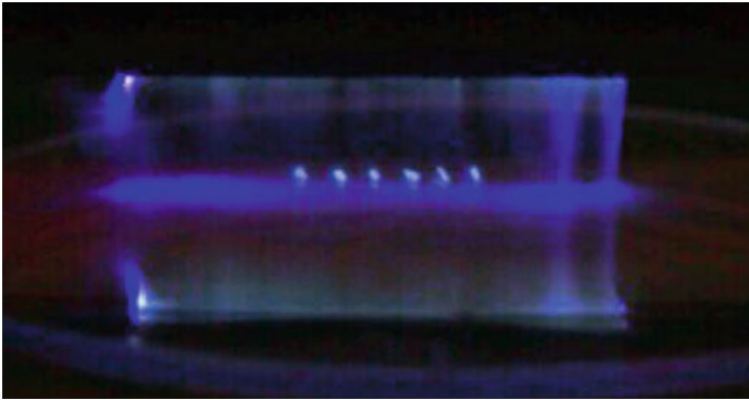
Fig. 12.8 A filamentary mode barrier discharge of Argon in air taken at PBP research center
