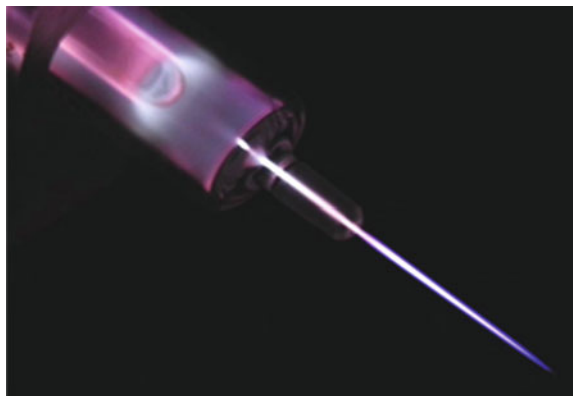
Fig. 12.2 A plasma needle operated at PBP research center
