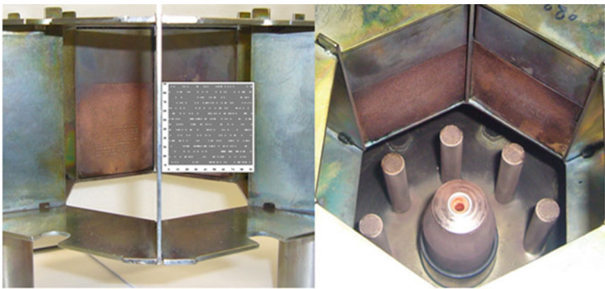
Fig. 6.36 Mask, its pattern and holder ( left ) and its position in front of anode top inside the plasma focus ( right ). [56]
