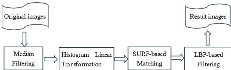
Fig. 1. The flow chart of the proposed E-SURF algorithm
