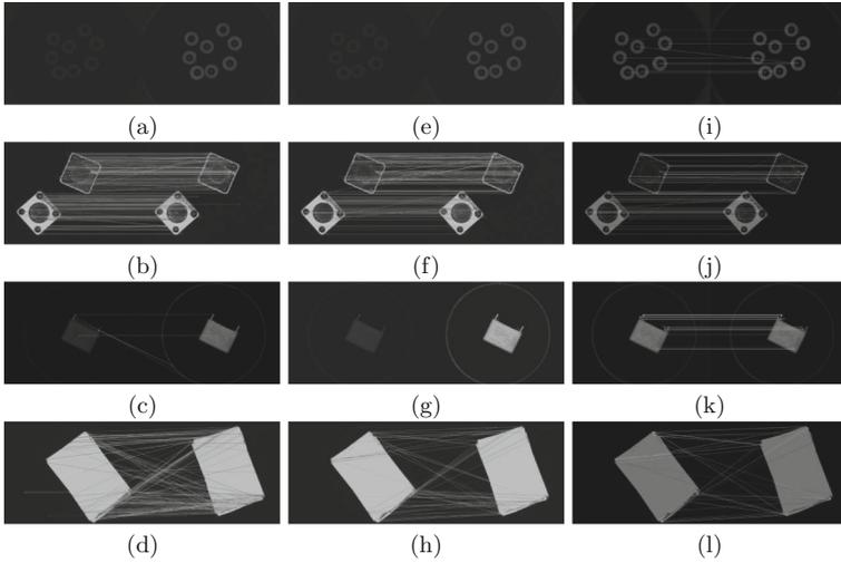
**Fig. 4.** Images from top to bottom: (a) (b) (c) (d) are matching results using original SIFT algorithm; (e) (f) (g) (h) are matching results using SURF algorithm; (i) (j) (k) (l) are results using SURF with pre-processing (Median Filtering and Histogram Linear Transformation)
