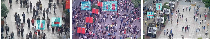
Fig. 10. The salient regions detection experimental results of the crowd saliency module.
