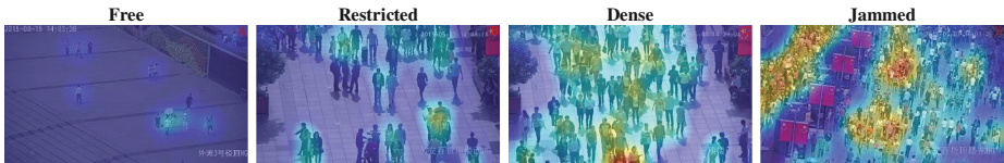
Fig. 8. The density distribution experimental results of the crowd density module.
