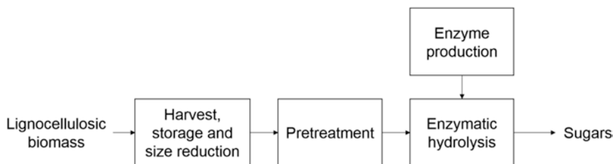
Fig. 1.2 Bioconversion process from lignocellulosic biomass to sugars
