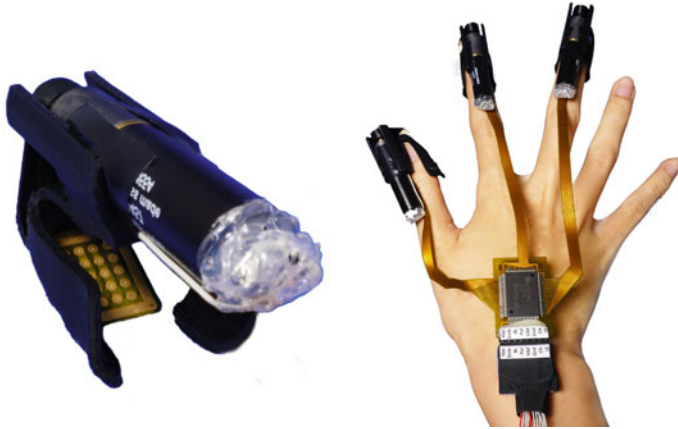
Fig. 2 FinGAR and photograph of device when worn on three fingers
