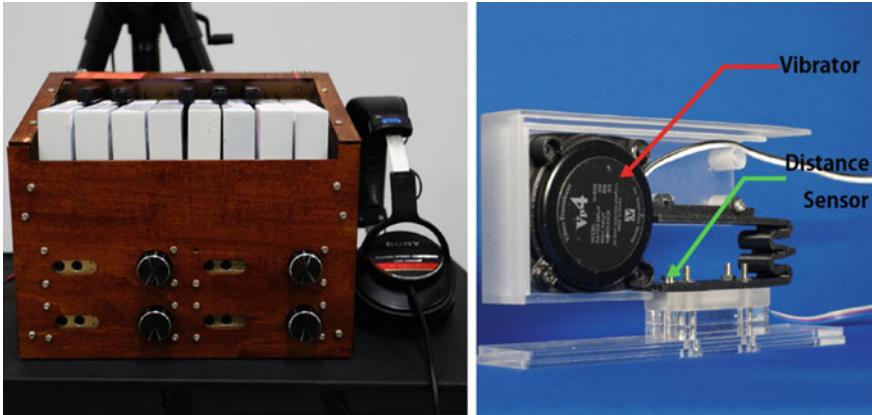
Fig. 1 HapTONE system (left) and the key unit (right)
