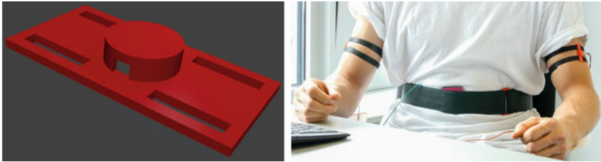
Fig. 2 3D model of tactor holder ( left ), user wearing attached tactors ( right )
