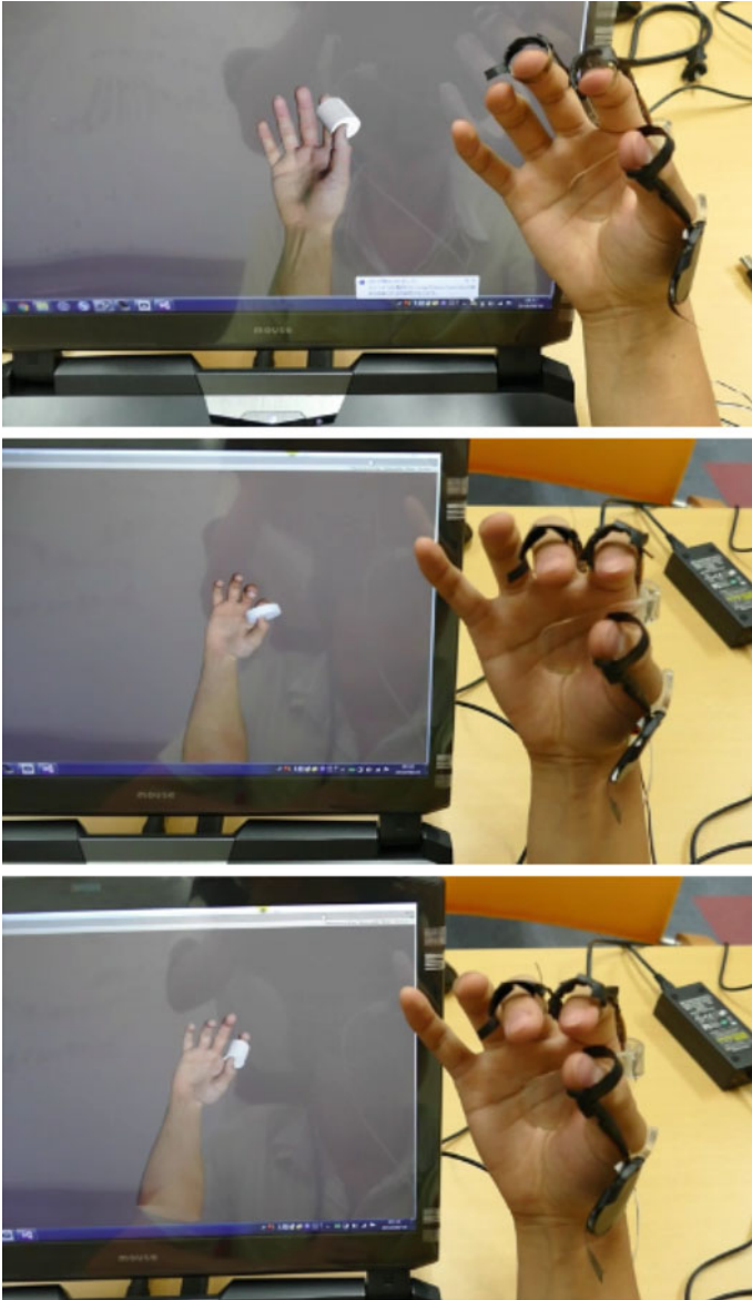
Fig. 3 Picture of re-rendered virtual hand displayed with its finger flexion unchanged ( top ), magnified ( middle ) and suppressed ( bottom )
