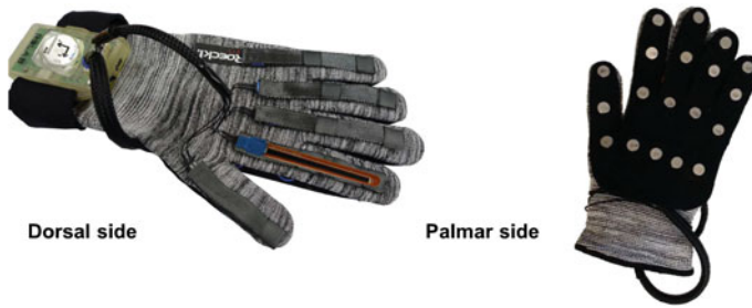
Fig. 1 Haptic Motion Glove, comprising of 19 vibration motors embedded in a soft layer on the palm, bend sensors on fingers, as well as control/communication/IMU modules attached near the wrist
