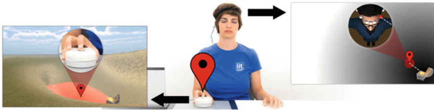
Fig. 3 The complementary feedbacks of our haptic system: vibrotactile HMD egocentric representation ( right ) and TAMO3 allocentric one ( left )
