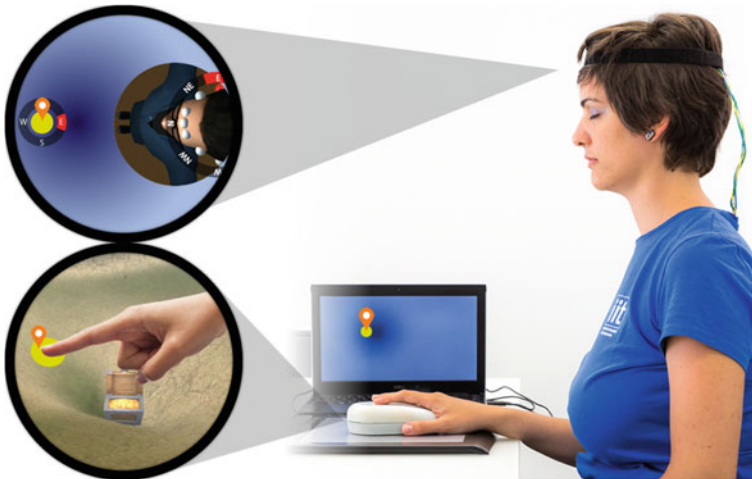
Fig. 2 Haptic system composed by the Tactile MOUSE 3 (TAMO3), and a vibrotactile HMD. While the TAMO3 supports the exploration of tactile maps from a top-view , the vibrotactile HMD provides an ego-references directional cue updated as a function of the TAMO3 movement
