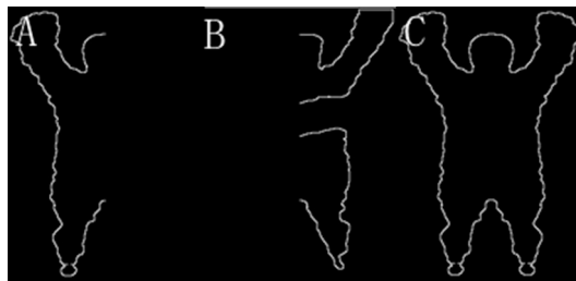
Fig. 6. The results of our contour extract algorithm. A: Left profile of human body. B: Right profile of human body. C: Full contour of human body.
