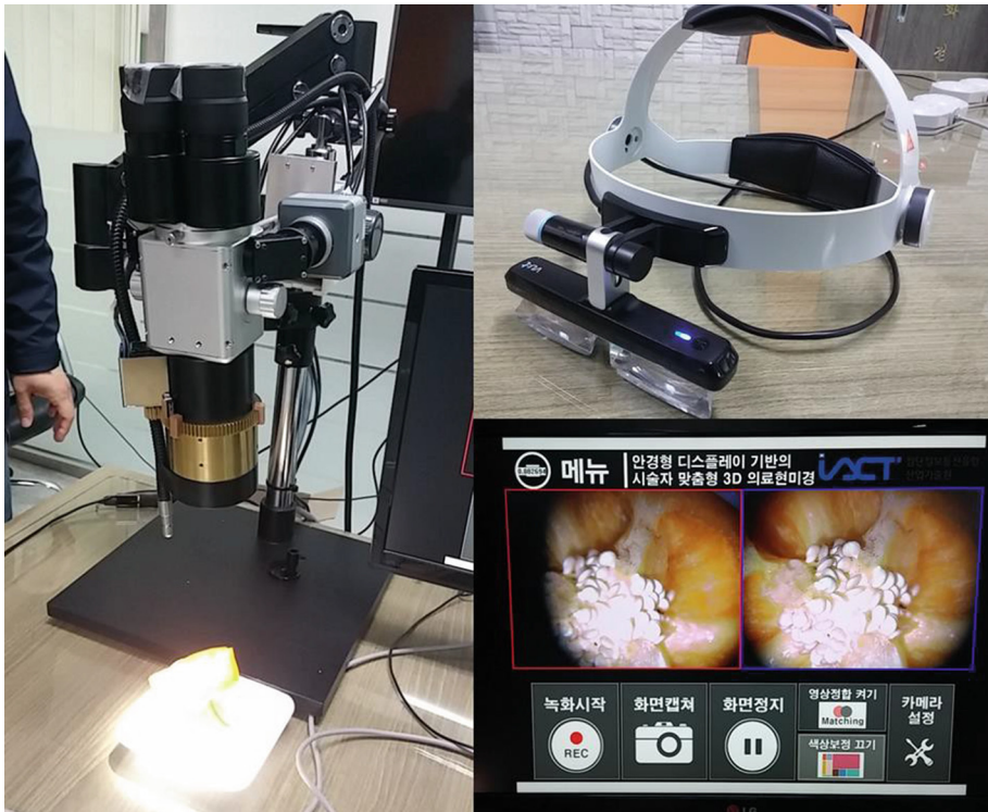
Fig. 4. 3D surgical microscope system with wireless HMD
