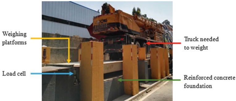
Fig. 7 The electric truck used to weight for trucks and materials. This is one of the applications by employing the evaluation method as a useful guidance for the product quality
