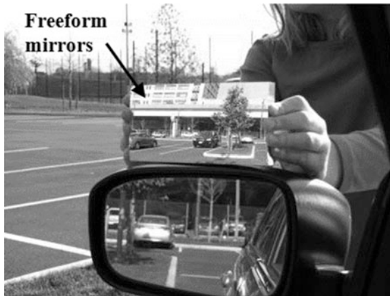
Fig. 1.4 Freeform reflector to eliminate the driver's blind spot effect [5]
