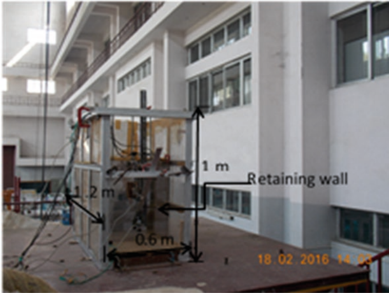
Fig. 25.3 Model container with typical model wall on shaking table
