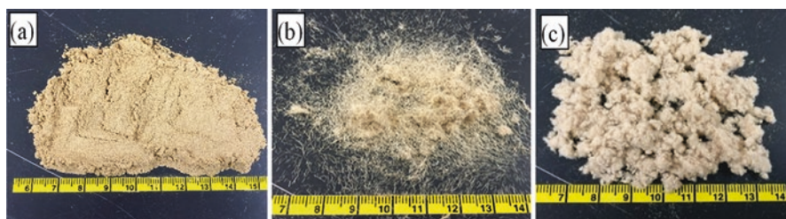
Fig. 9.2 Cellulose adsorbents: (a) peanut hulls, (b) jute fibers, and (c) kraft pulp
