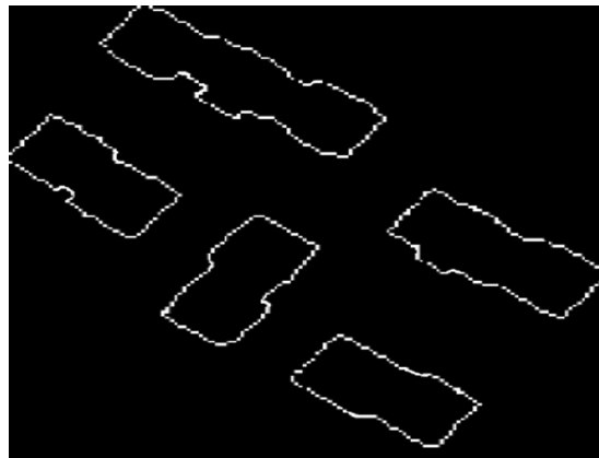
Fig. 10. The effect of detection using Sobel operator
