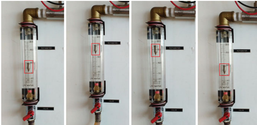
Fig. 3 Rotameter float is at different positions sensed by camera and calibrated in terms of level
