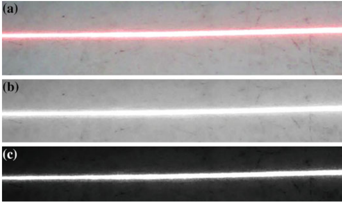
Fig. 3 a Laser line image. b Grayscale conversion of above image. c Image enhancement using exponential lookup table
