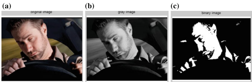
Fig. 3 a Original image. b Grey-scale image. c Binary image
