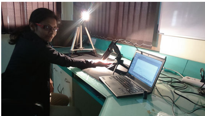
Fig. 3 Laboratory experimental measurement setup of palmprint Spectra
