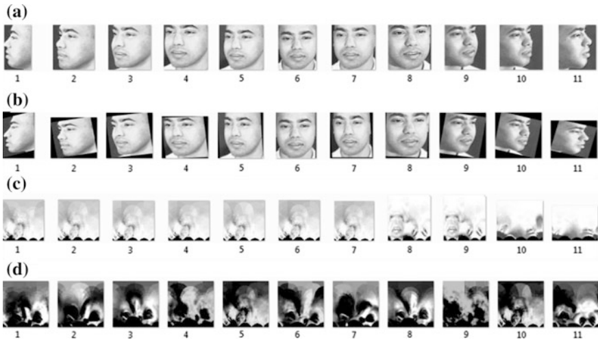
Fig. 2 Steps showing sample images from IRIS face database after a masking, b registration, c log-polar transformation, d eigenfaces
