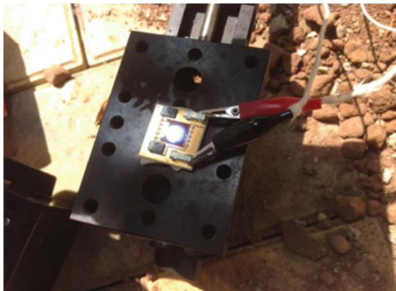
Fig. 2 A Multi-junction concentrator cell under white light illumination
