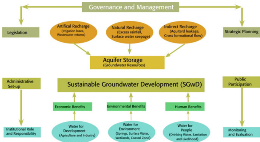
Fig. 42.6 Conceptual approach to achieve sustainable groundwater development balancing recharge inputs to aquifer storage plus change in storage against discharge outputs (Adapted from Hiscock et al. 2002)
