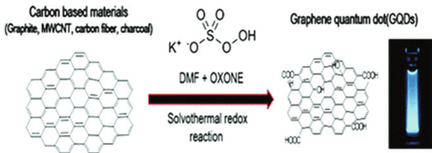
Fig. 4.15 Mechanism of GQDs synthesis by solvothermal method. Reprinted with permission from Ref. [49]. Copyright 2015, Royal Society of Chemistry
