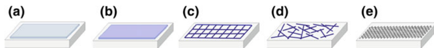
Fig. 5.1 An illustration of transparent conductive films composed of different materials: a ITO metal oxide, b conductive polymer, c periodic metal grid, d percolated random network of one-dimensional nanostructures, such as carbon nanotubes and metal nanowires, and e two-dimensional graphene
