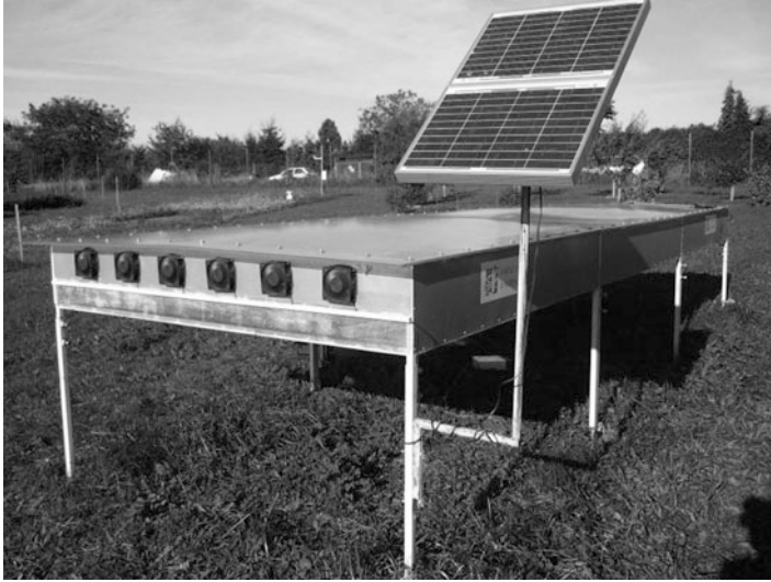
Fig. 19 The double-pass solar dryer installed at the experimental field of Czech University of Life Sciences Prague (Kucerova et al. 2015)
