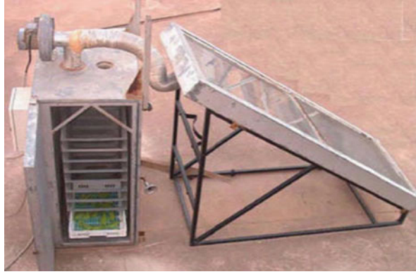
Fig. 5 Indirect solar dryer (Prakash et al. 2016)
