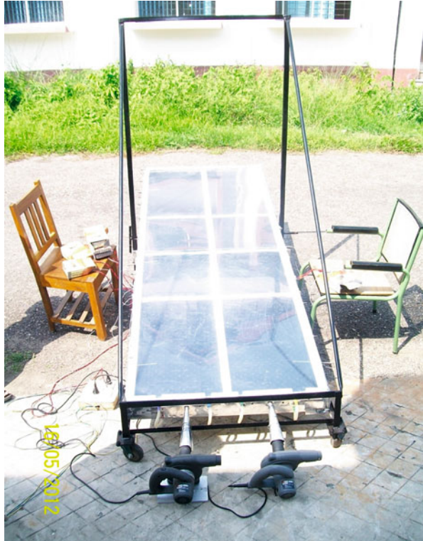
Fig. 6 Improved solar air heater: experimental setup
