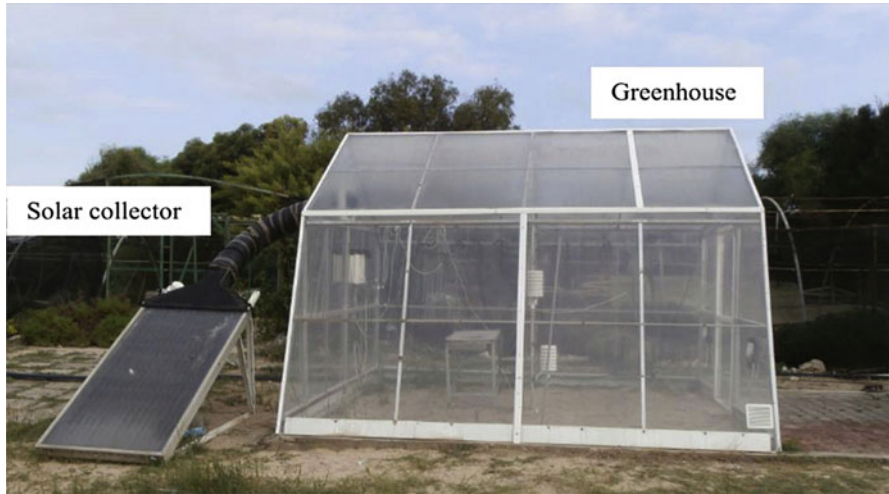
Fig. 8 Photograph of mixed-mode-type solar greenhouse dryer (Elkhadraoui et al. 2015)
