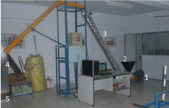
Fig. 6 Experimental setup for testing using heated pipe (Kamaruddin et al. 2014)
