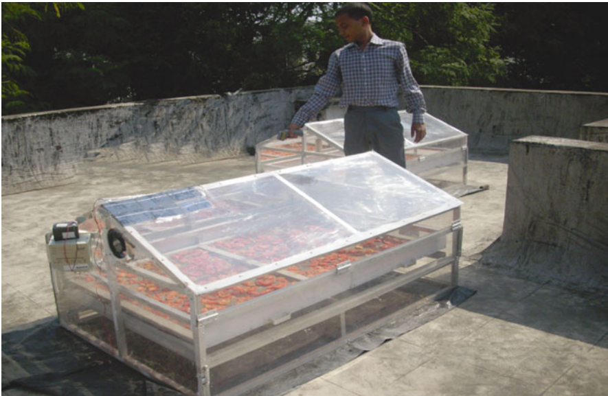
Fig. 1 Photograph of active mode modified greenhouse dryer (Prakash and Kumar 2014)
