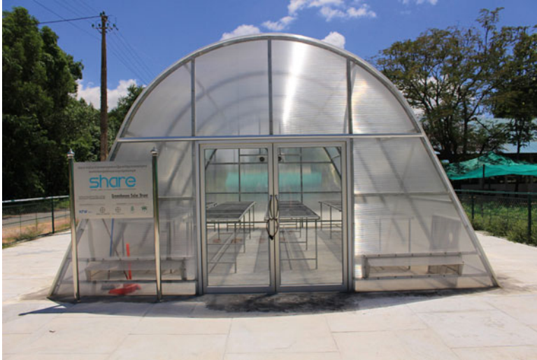
Fig. 13 Solar greenhouse dryer installed at the Royal University of Agriculture in Cambodia (Photo: J. Banout)
