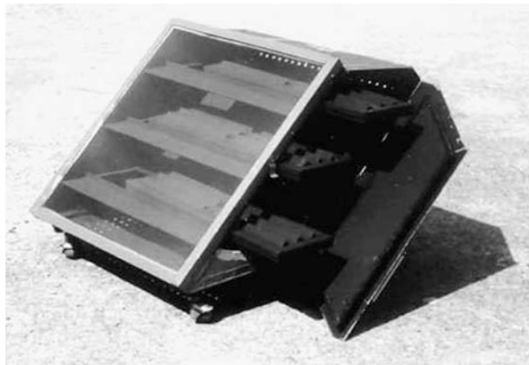
Fig. 8 Photograph of PAU domestic solar dryer with open doors (Singh et al. 2006)
