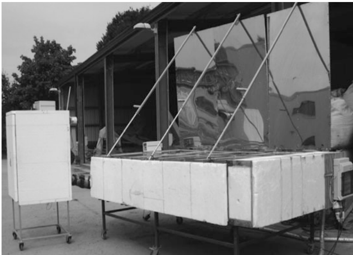
Fig. 7 Hybrid solar dryer (Chauhan et al. 2015)
