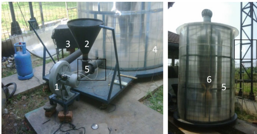
Fig. 25 Blower (1), feed hopper (2), LPG stove (3), transparent structure (4), pneumatic conveyor (5), and receiving hopper (6) (Nining 2015)
