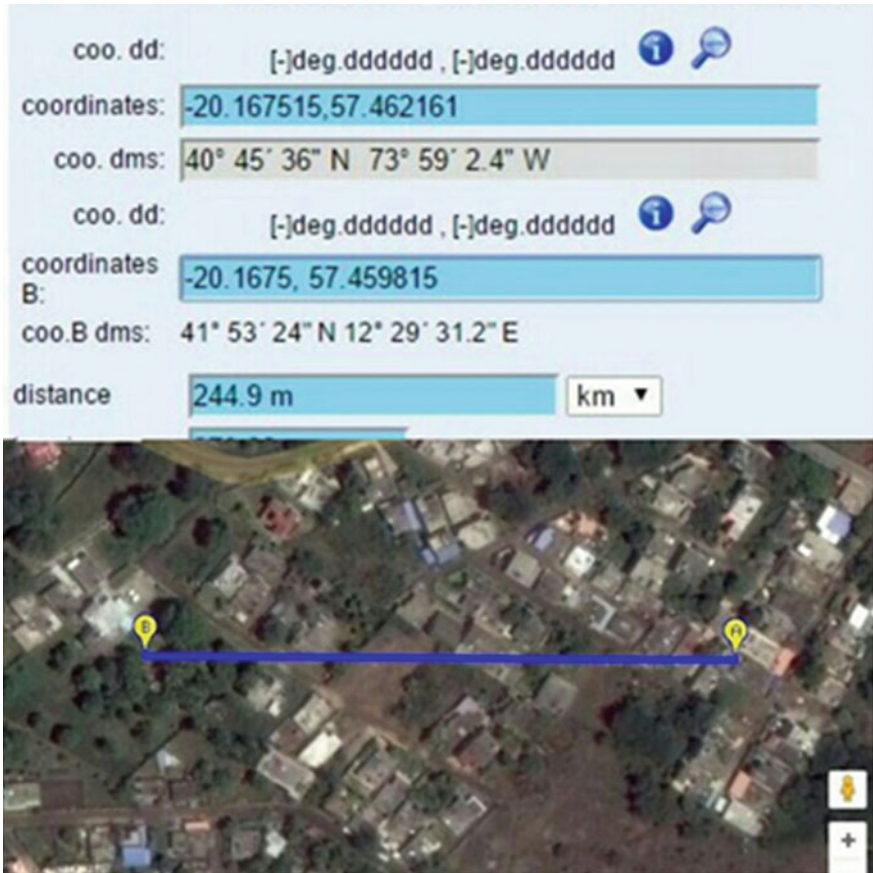
Fig. 3 Link length measurement using Sun–Earth tools
