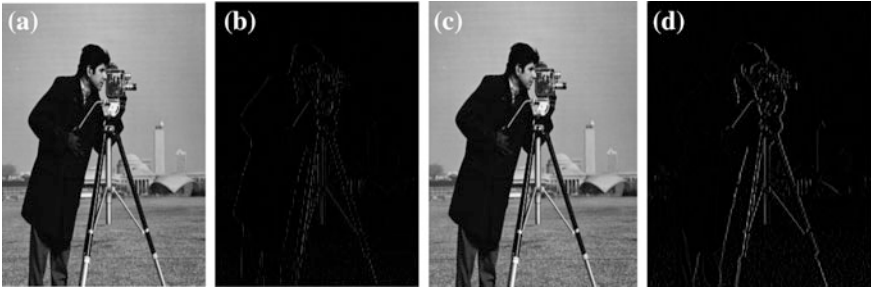
Fig. 3 a Reconstructed image. b Error image obtained using proposed technique. c Reconstructed image. d Error image obtained using DWT technique for camera man image
