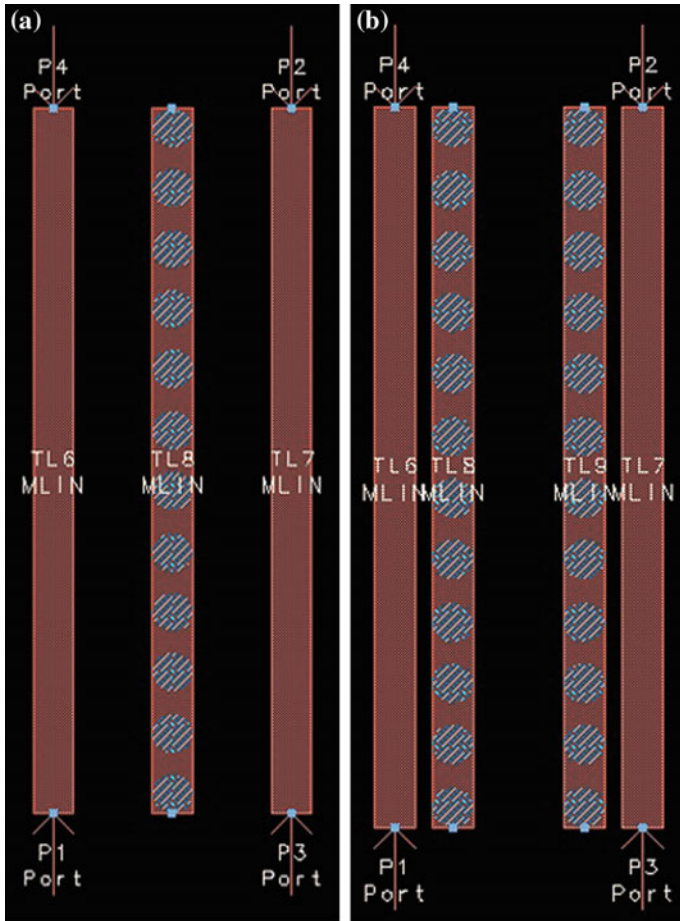
Fig. 4 Layout of two transmission lines with vias on a Single trace. b Two
