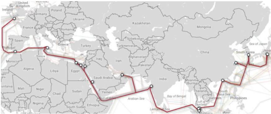
Fig. 2 Topology of Flag Europe-Asia undersea cable network. It has 16 nodes or cable landing points in Europe and Asia
