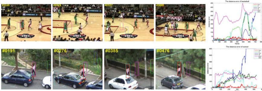
Fig. 2 Examples of the tracking results on Basketball (1st row) and Woman (2nd row) sequences. The predicted bounding boxes of the six trackers are presented with different colors: Ours (red), CT (green), CSK (blue), VR (black), BSBT (purple) and SMS (cyan). The CLE plots of each frame are shown in the last column. Best viewed on a high-resolution screen. (Color figure online)
