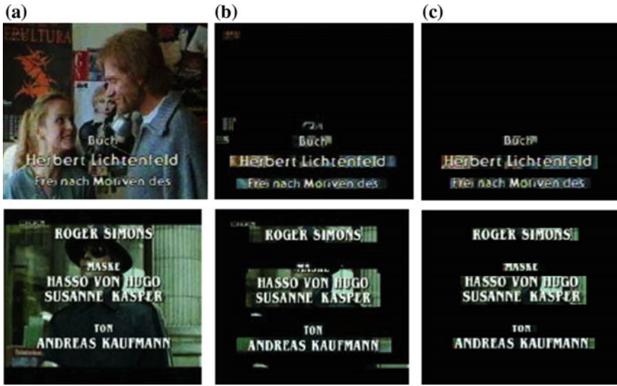
Fig. 4 Comparison of the extracted text regions. a Original image. b Extracted caption text regions by the method of Ref. [7]. c Extracted caption text regions by our method
