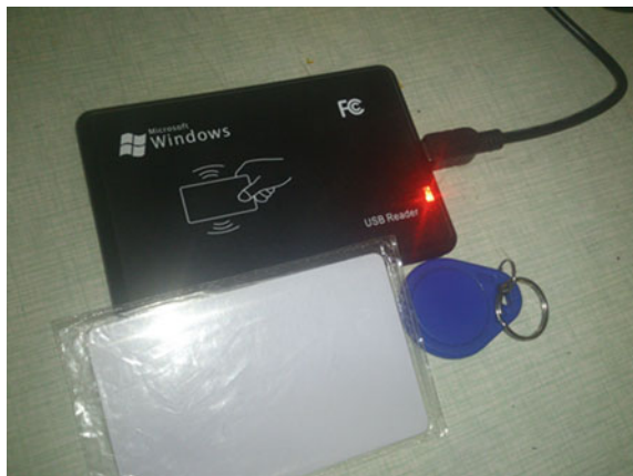
Fig. 2 RFID read and write device
