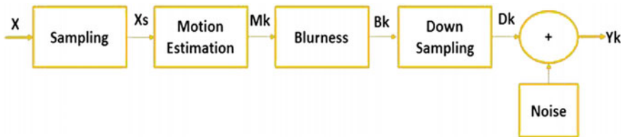
Fig. 3 Observation model of super resolution
