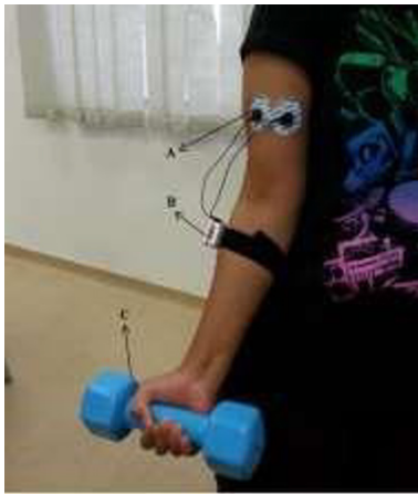
Fig 1 Experimental protocol setup. A) electrode placed on BB muscle, B) wireless EMG sensor, C) a 3-kg dumbbell.
