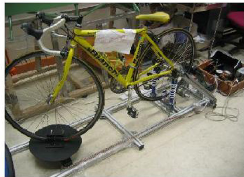
Fig. 6. Arrangement of virtual reality cycling simulator [10]
