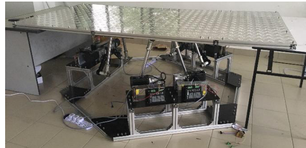
Fig. 4. Actual scale prototype of 6DOF platform
