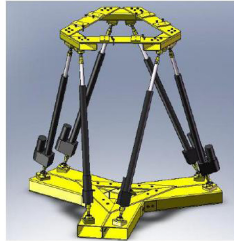
Fig. 3. Example of the 6 DOF Motion platform based on Stewart Platform design. [4]
