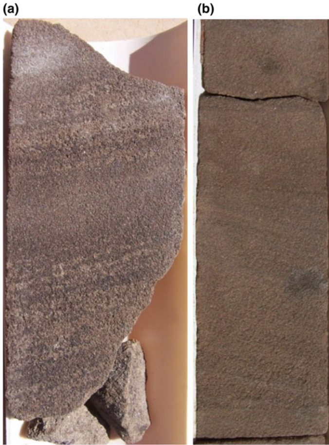
Fig. 5 Trough cross-stratified sandstone, a core three well HE 28 at depth (1660.30–1660.40) b core two well HE 38 at depth (1645.20–1645.50)
