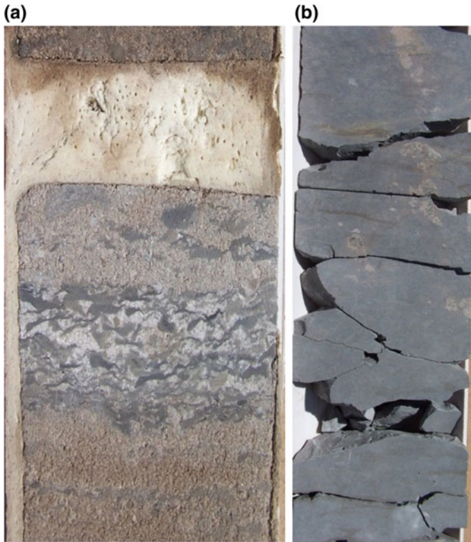
Fig. 7 Mudstone facies: layered mudstone a well HE 28 core 1 depth 1638.25 and massive mudstone b well HE core 3 depth 1654.55–1655.00
