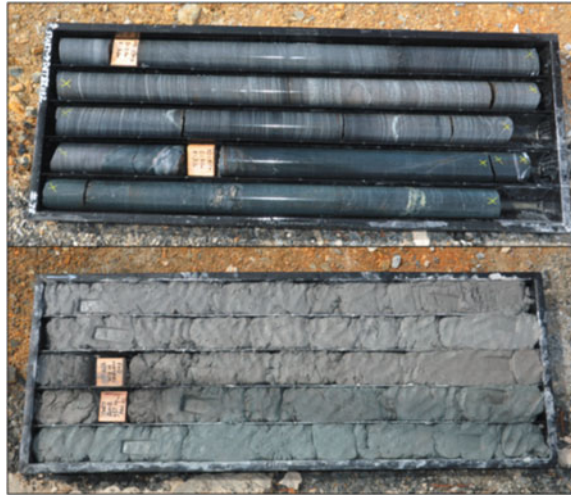
Fig. 2 Brukunga core and corresponding cuttings by diamond-impregnated drill bit collected and packed in sequence (DET CRC eNewsletter July 2013)
