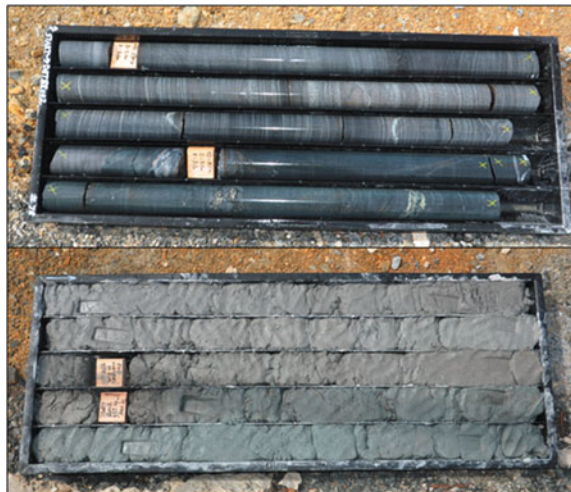
Fig. 2 Core samples ( top ) and drilled hard rock cuttings ( bottom ) by diamond-impregnated drill bit
