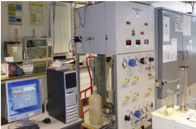
Fig. 2 High-temperature high-pressure (HTHP) relative permeability system for the MRF experiments
