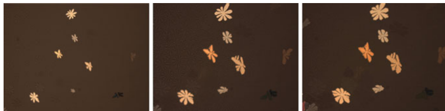
Fig. 3 Textures observed at 120 °C ( left ), 100 °C ( center ) and room temperature ( right ) during cooling process
