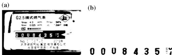
Fig. 1 a Gas meter images before location process and b gas meter images after location process
