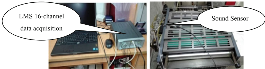
Fig. 4 The experimental platform of press sound signal acquisition
