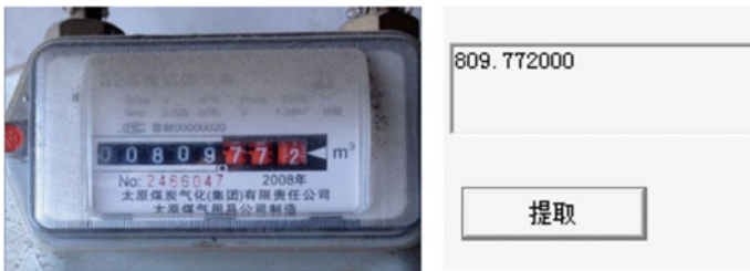
Fig. 5 Gas meter images and recognition results
