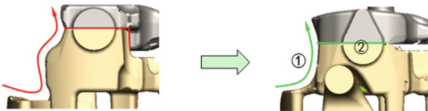
Fig. 16.4 Main structure optimization scheme of water jacket
