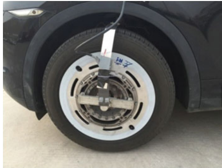
Fig. 3.4 Acceleration acquisition from road test
