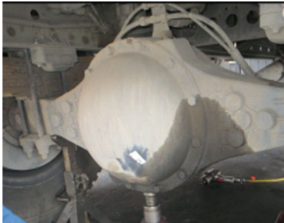
Fig. 35.11 Lower right oil leakage
