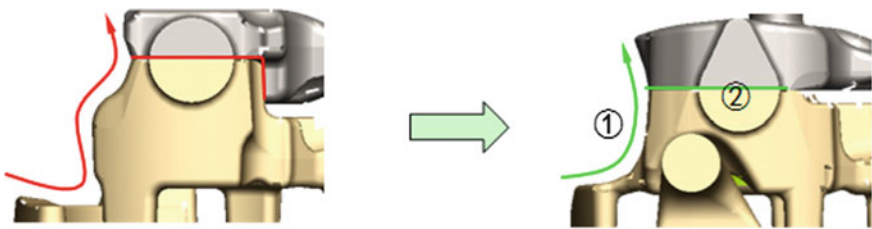
Fig. 16.4 Main structure optimization scheme of water jacket
