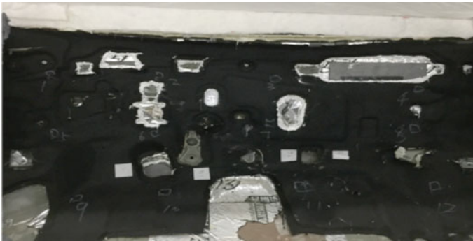
Fig. 34.3 Inner dash test between the reverberation and anechoic chamber
