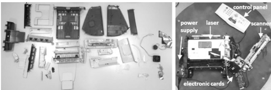
Fig. 2 Removed parts; living product after autopsy
