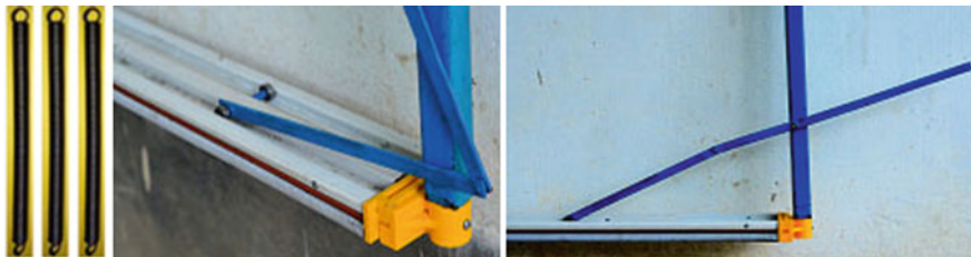
Fig. 9 Iron suspension inside the holding pipe ( image-1 ); Magnet bearing shaft with holding assembly pipe ( image-2 ); Sliding lever of magnet bearing shaft ( image-3 ) ( Source Site pictures of Deepak's innovation)
