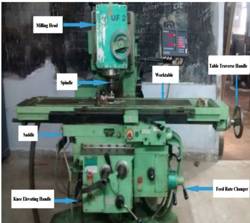
Fig. 2 Experimental set up for end milling operation
