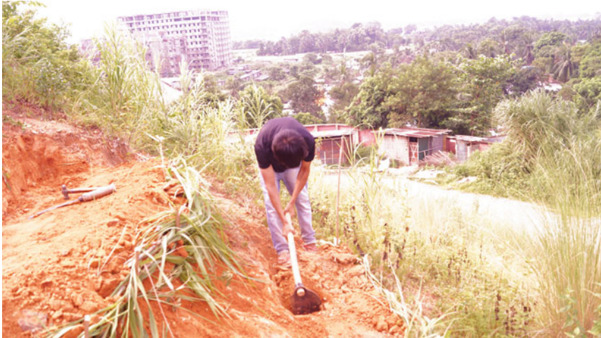
Fig. 3 Digging in horizontal direction with the modified spade
