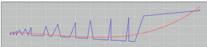
Fig. 4 An example of polynomial smoothing on a jerky pointing movement. The red line is the smoothed line, and the blue line is the original movement
