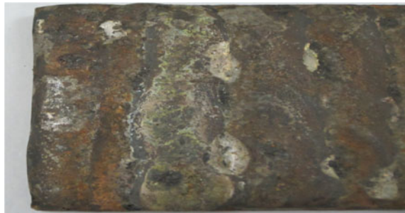
Fig. 2 Hardfacing coating after welding
